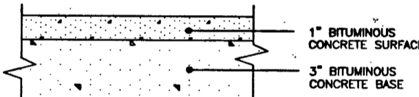
FULL DEPTH BIT. CONC. ALTERNATIVE P-1 PAVING DETAIL NOT TO SCALE
