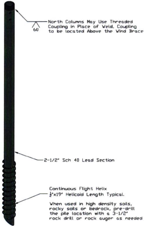
Helical Pile Detail
