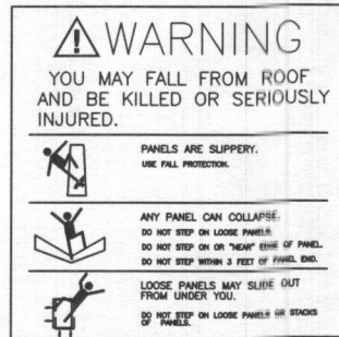
Roof Panel Warning
