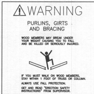
Wood Member Warning
