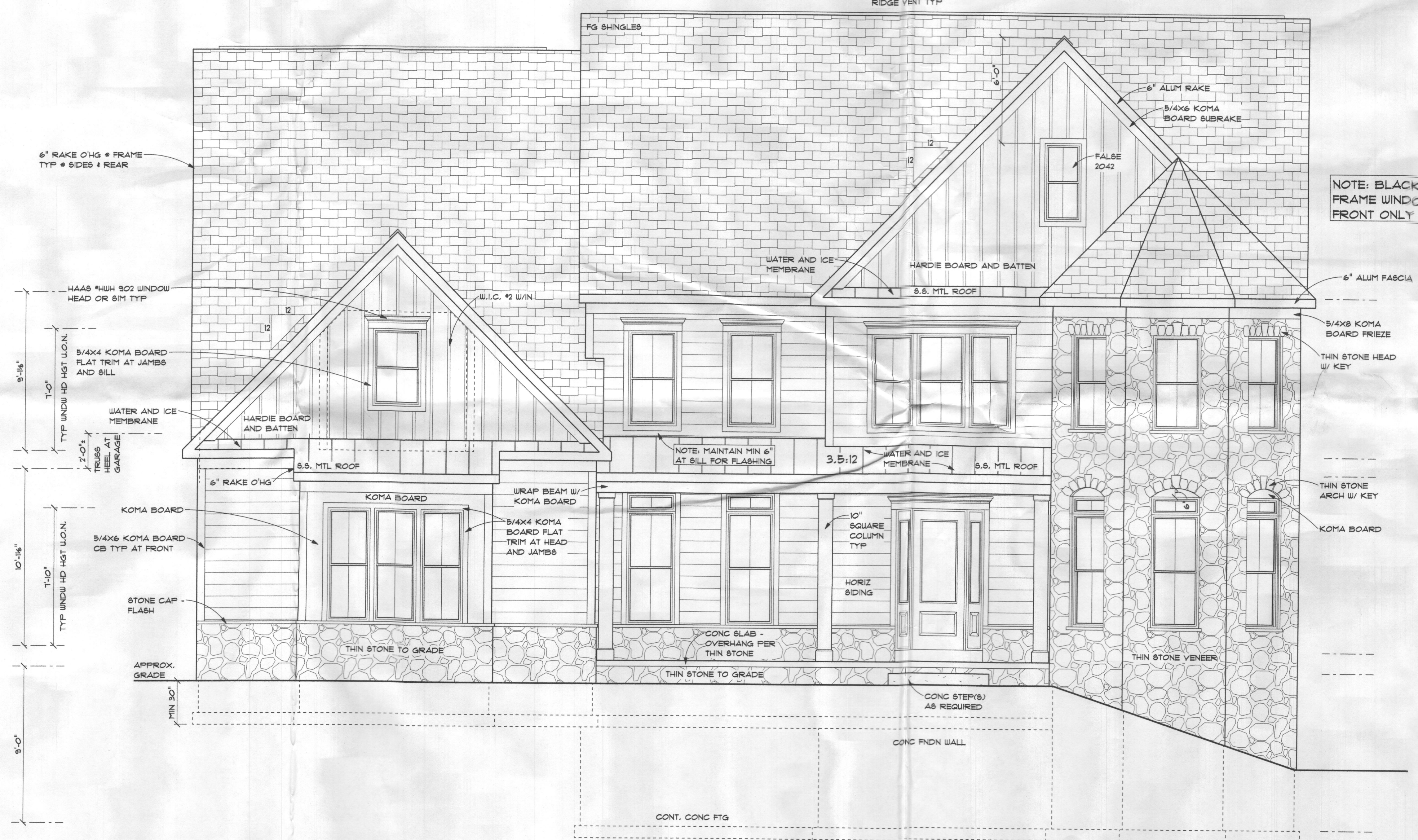
Front Elevation #805 SCALE: 1/4" = 1'-0"
