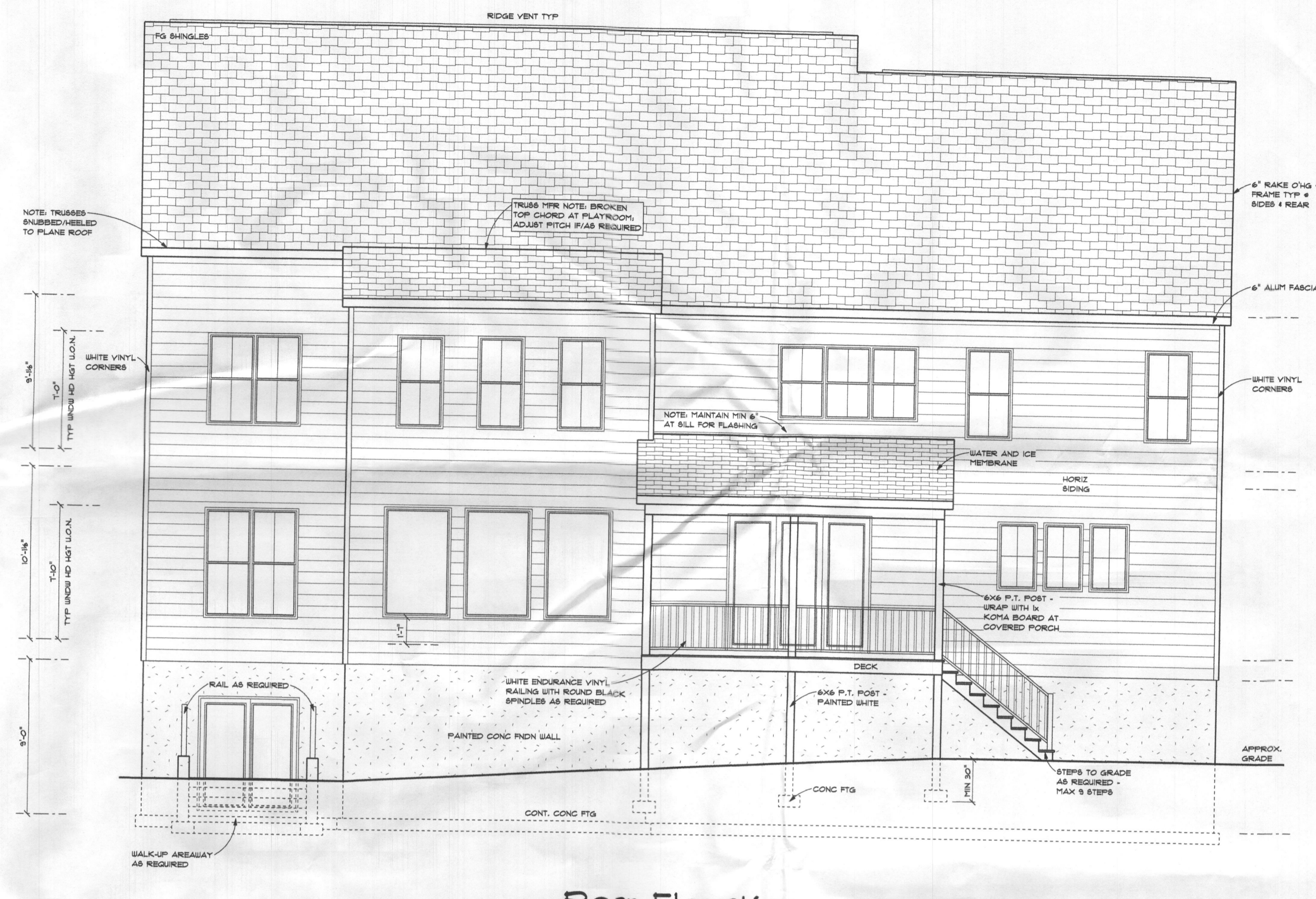
Rear Elevation SCALE: 3/16" = 1'-0"
