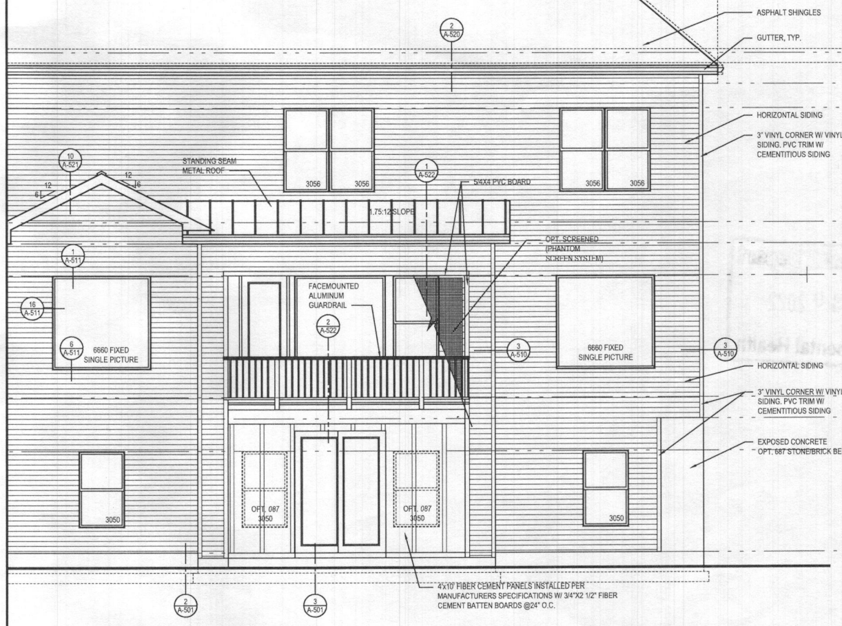
4 REAR ELEVATION w/ OPT. 263169 - COV'D OUTDOOR LIVING @ WALKOUT CONDITION A-403 SCALE: 1/4"=1'-0" TOL081A_A403.DWG
