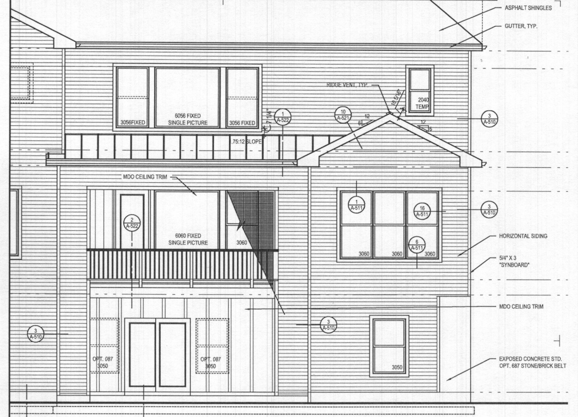
4 REAR ELEVATION w/ OPT. 263073 MULTI-GEN. SUITE A-407 SCALE: 1/4"=1'-0" TOL081A_A407.DWG w/ COVD OUTDOOR LIVING @ WALKOUT CONDITION
