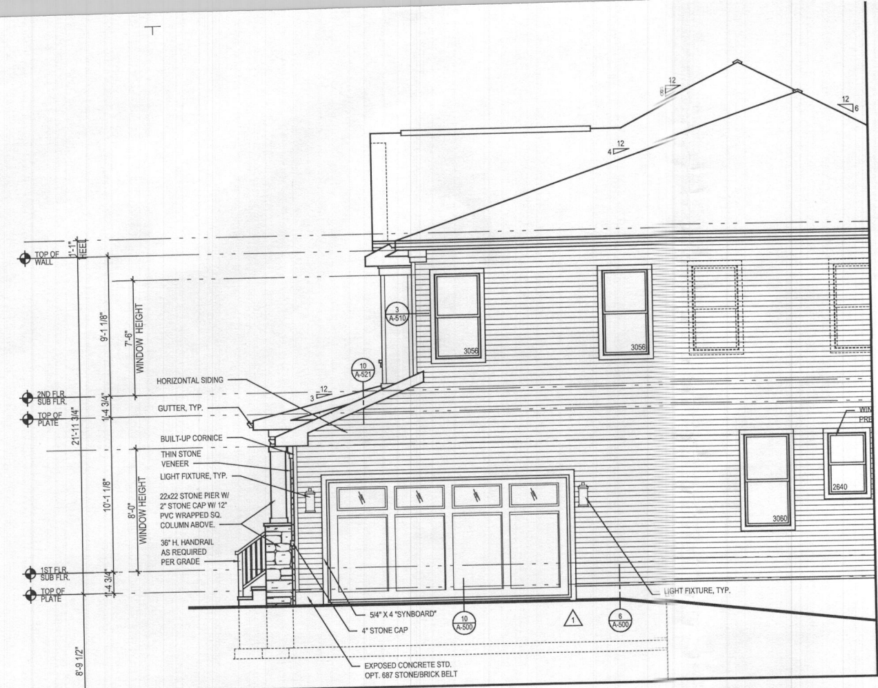
4 PART. RIGHT SIDE ELEVATION w/ OPT. 012 - SIDE LOAD GARAGE ELEV. 1 - SHOWN A-400 SCALE: 1/4"=1'-0" TOL081A_A400.DWG
