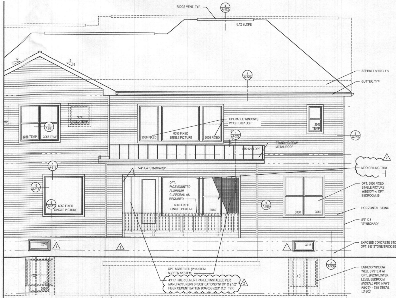
4 REAR ELEVATION w/ OPT. 263165 - LUXURY OUTDOOR LIVING @ BURIED CONDITION A-402 SCALE: 1/4"=1'-0" TOL081a_A402.DWG
