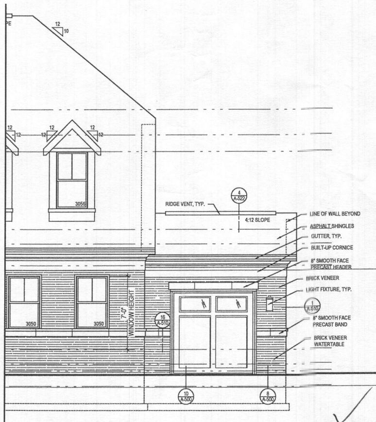
2 PART. FRONT ELEV. w/ OPT. 263102 - ONE CAR FRONT ENTRY GARAGE A-401a SCALE: 1/4"=1'-0" TOLB19C_A401.DWG TRADITIONAL *SHOWN W/ OPT. SIDE LOAD GARGE, TYP.
