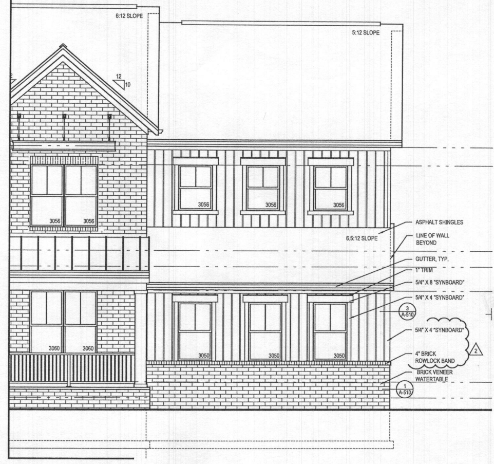
3 PART. FRONT ELEVATION w/ OPT. 012 - SIDE LOAD GARAGE A-400d SCALE: 1/4"=1'-0" TOLUBA_ARCH.DWG ELEV. 5 - SHOWN
