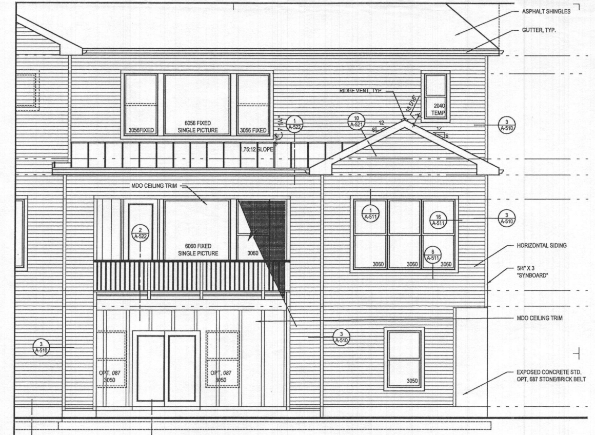
4 REAR ELEVATION A-407 SCALE: 1/4"=1'-0" w/ OPT. 263073 MULTI-GEN. SUITE w/ COVID OUTDOOR LIVING @ WALKOUT CONDITION
