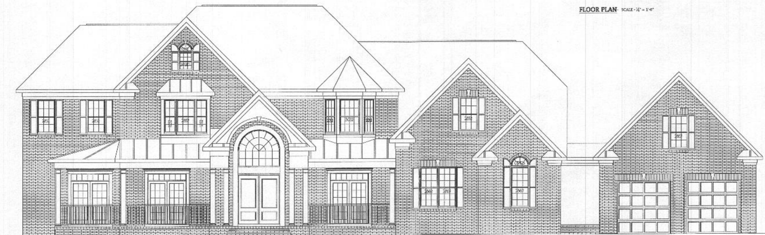
FRONT ELEVATION - SHOWN W/ OPT. CONSERVATORY, BRICK FRONT, ANGLED PORCH AND DETACHED GARAGE. SCALE - 1/2" = 1'-0"
