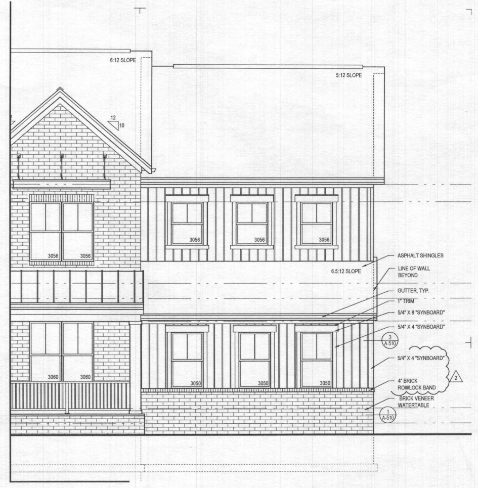
3 PART. FRONT ELEVATION w/ OPT. 012 - SIDE LOAD GARAGE ELEV. 5 - SHOWN SCALE: 1/4"=1'-0" TOL081A_A400.DWG
