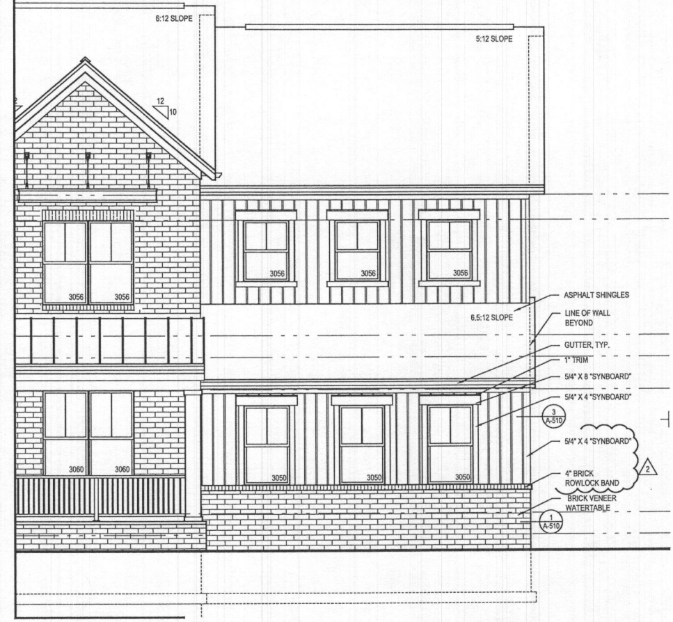
3 PART. FRONT ELEVATION w/ OPT. 012 - SIDE LOAD GARAGE ELEV. 5 - SHOWN SCALE: 1/4"=1'-0" TOL081A_A400.DWG
