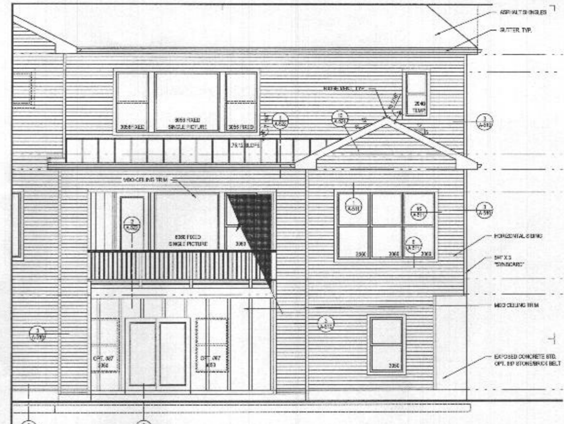
4 REAR ELEVATION A-407 SCALE 1/4"=1'-0" w/ OPT. 263073 MULTI-GEN. SUITE w/ OPT. OUTDOOR LIVING @ WALKOUT CONDITION
