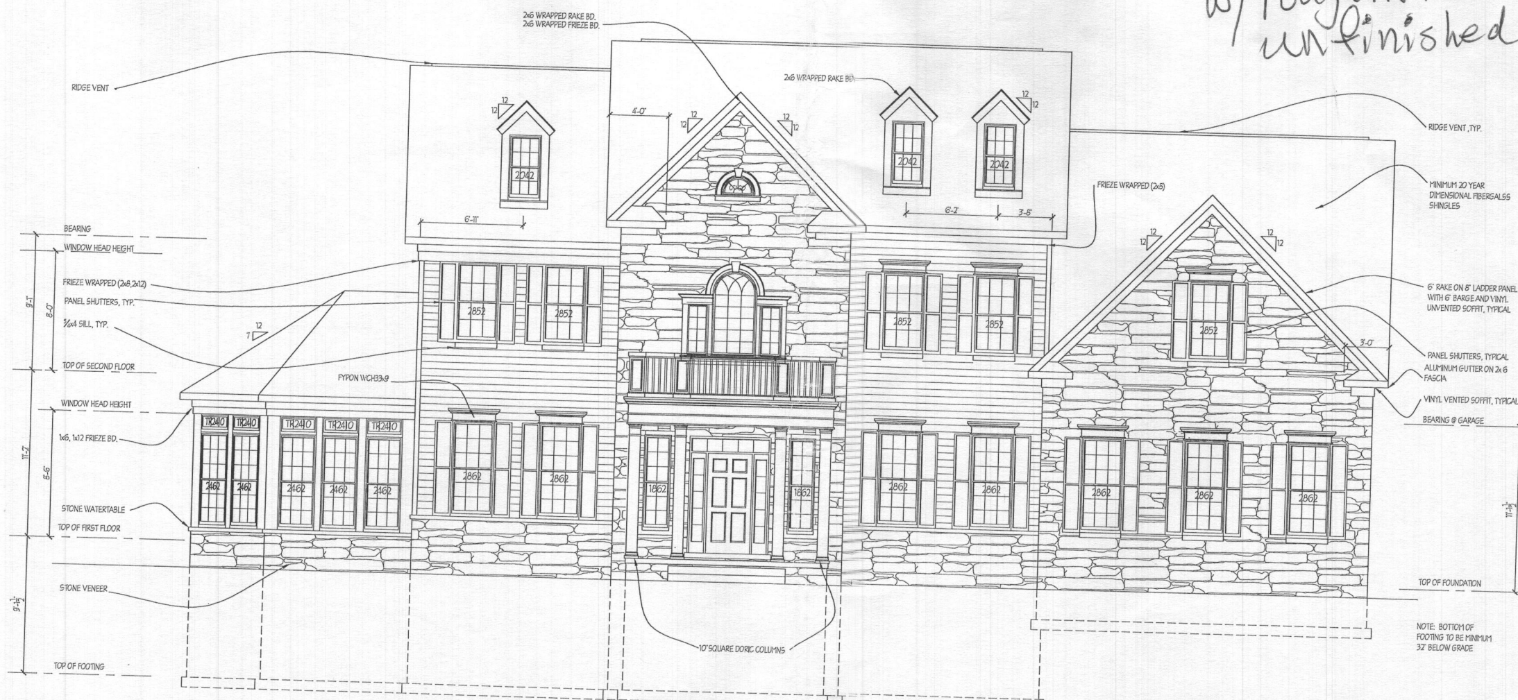
FRONT ELEVATION #6 SHOWN W/OPT. CONSERVATORY AND STONE PORCH SCALE: 1/4" = 1'-0"
