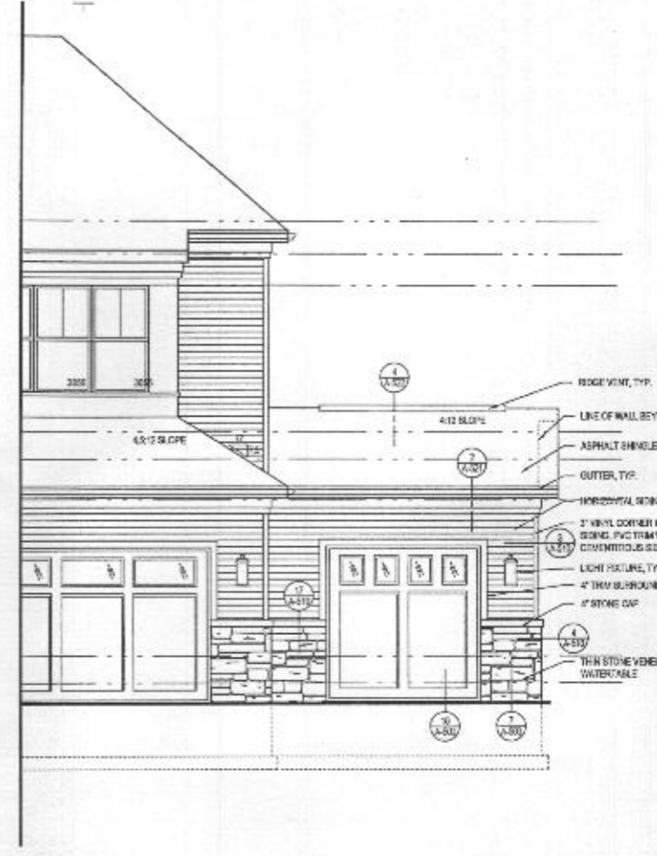
4 PART. FRONT ELEVATION w/ OPT. 263102 - ONE CAR GARAGE A-401 SCALE 1/4"=1'-0" ELEV. 1 - CRAFTSMAN - SHOWN
