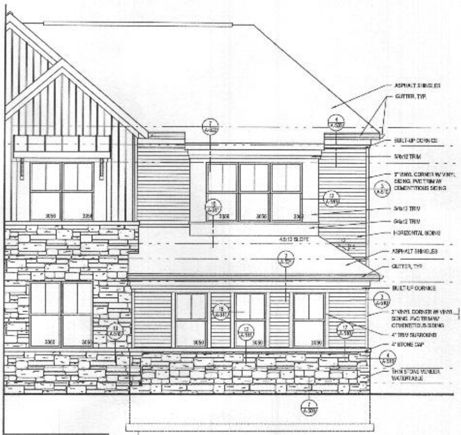
3 PART. FRONT ELEVATION w/ OPT. 012 - SIDE LOAD GARAGE SCALE: 1/4"=1'-0" ELEV. 1 - CRAFTSMAN - SHOWN
