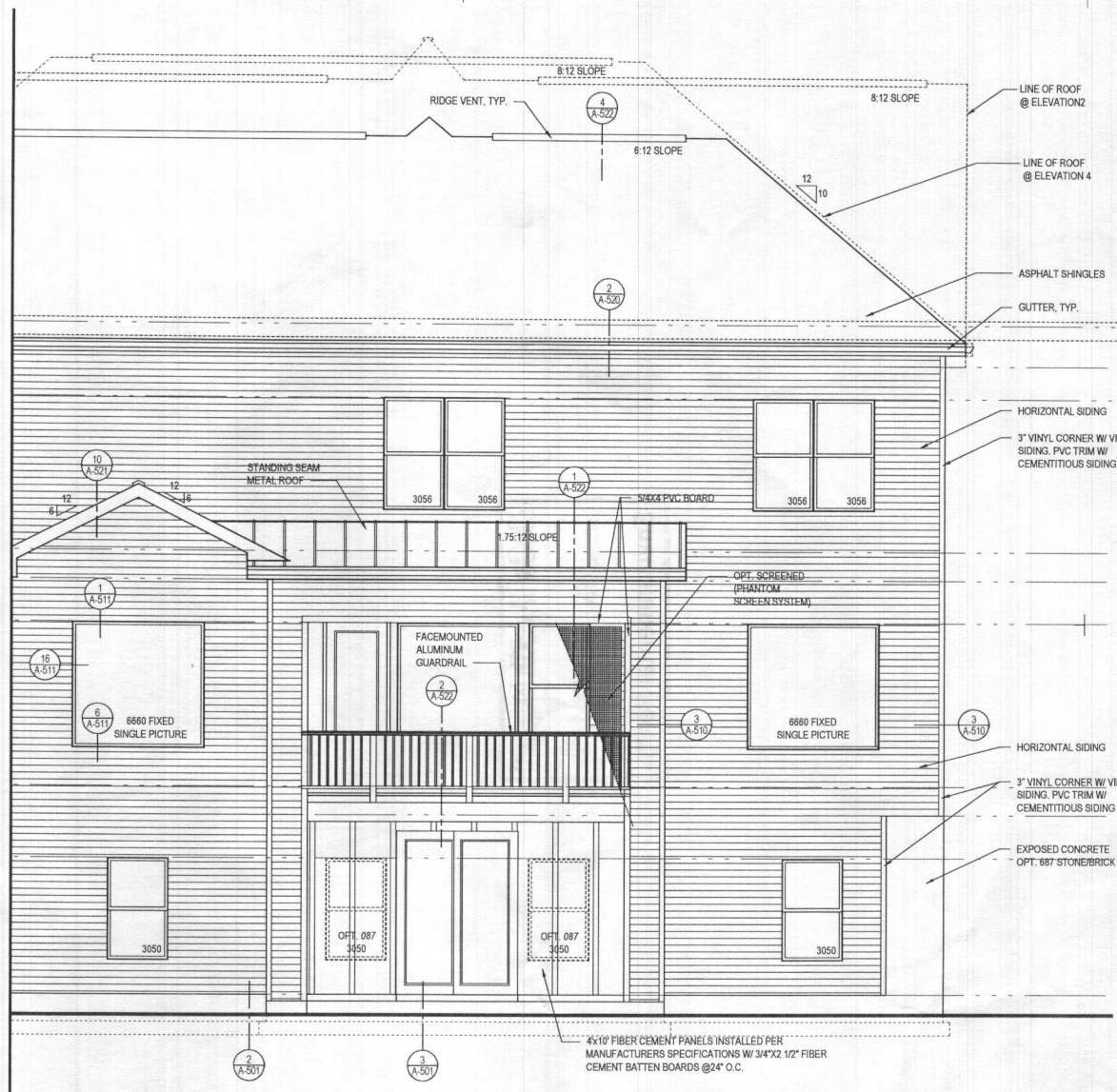
4 REAR ELEVATION w/ OPT. 263169 - COVD OUTDOOR LIVING @ WALKOUT CONDITION SCALE: 1/4"=1'-0" TOL081A_A403.DWG
