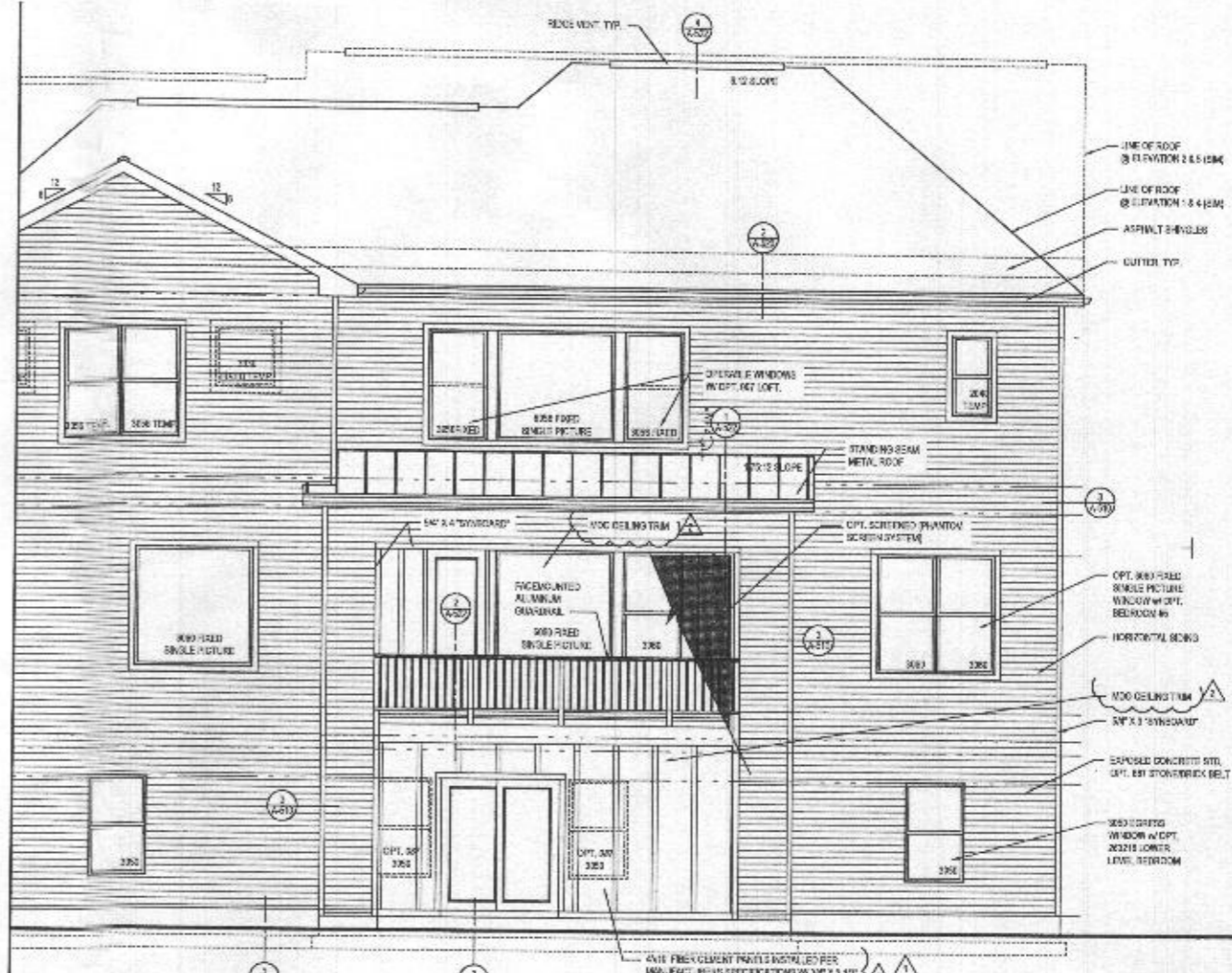
4 REAR ELEVATION A-403 SCALE: 1/4"=1'-0" TYPICAL WALLS
