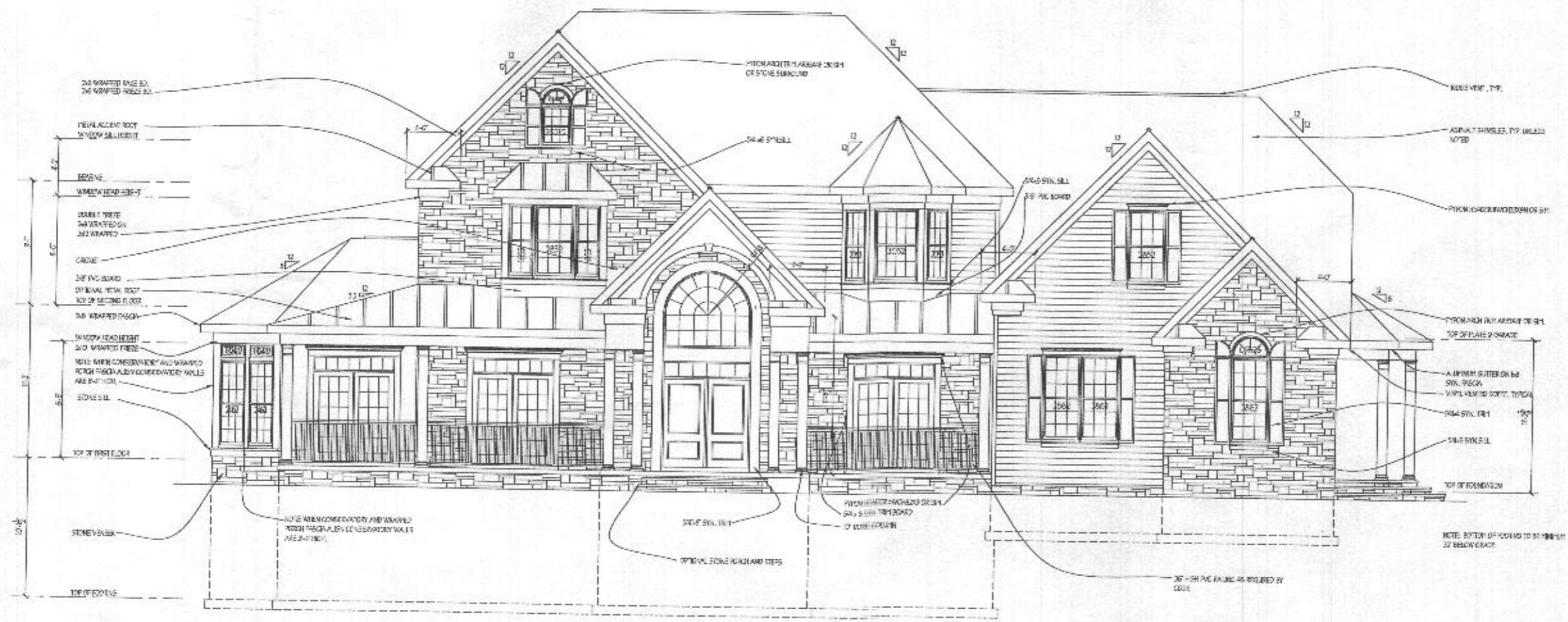
FRONT ELEVATION - SHOWN W/ OPT. CONSERVATORY AND SIDE PORCH SCALE: 1/4" = 1'-0"
