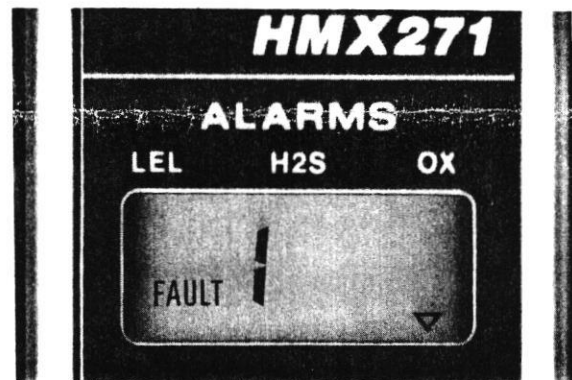
If the instrument's combustible gas sensor should malfunction, the monitor will go into a failure mode similar to the low battery failure mode. The word "FAULT" will appear in the lower left corner of this display, and the audible alarm will sound a continuous tone.
