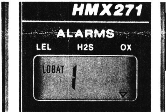
In the battery failure mode, the LCD becomes blank except for the numeral "1" and the word "LOBAT", and the audible alarm sounds a continuous tone. Approximately 1/2 hour before this condition, the audible alarm begins to beep periodically, with the time between beeps decreasing, as the battery nears the end of its useful charge life.
