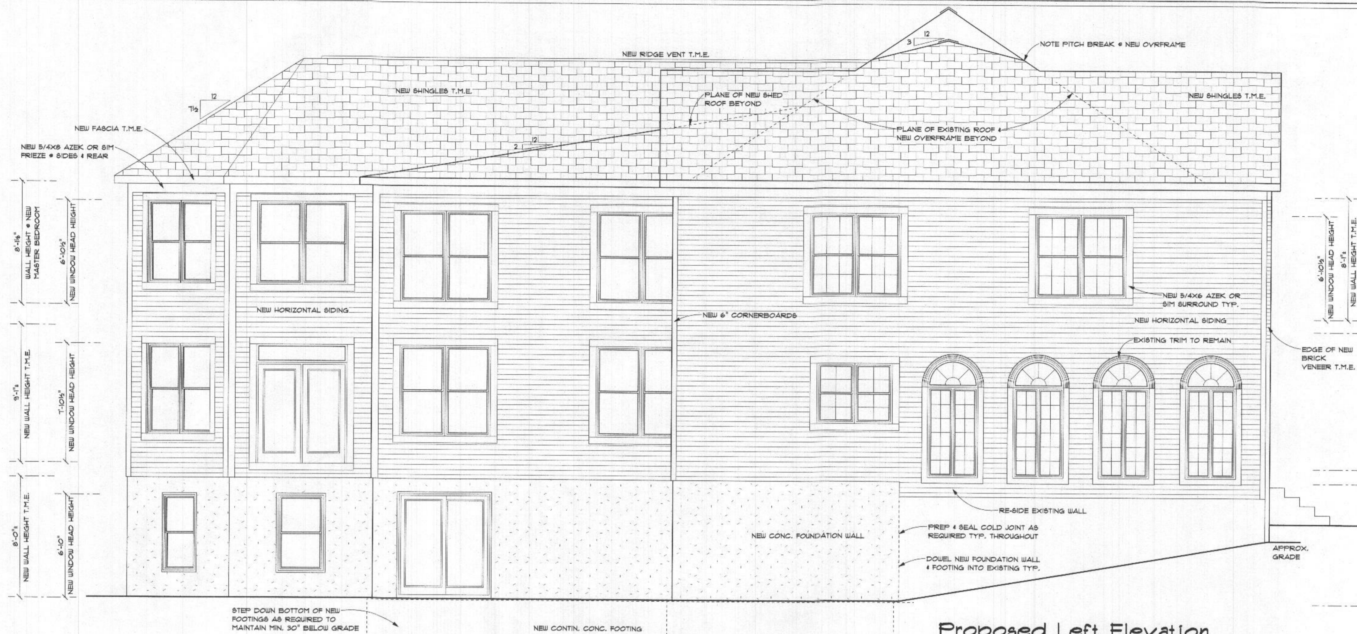
Proposed Left Elevation SCALE: 1/4" = 1'-0"
