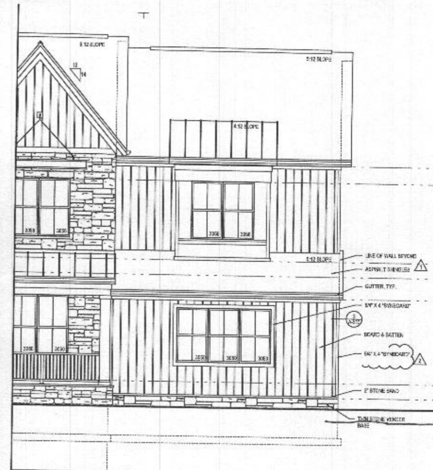
3 PART. FRONT ELEVATION w/ OPT. 012 - SIDE LOAD GARAGE A-400b SCALE: 1/4"=1'-0" ELEV. 2 - SHOWN
