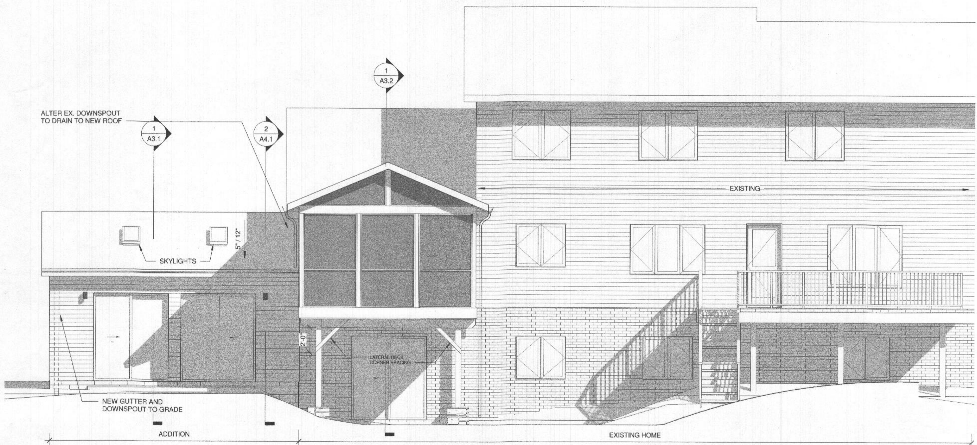
2 Rear Elevation - Addition 1/4" = 1'-0"
