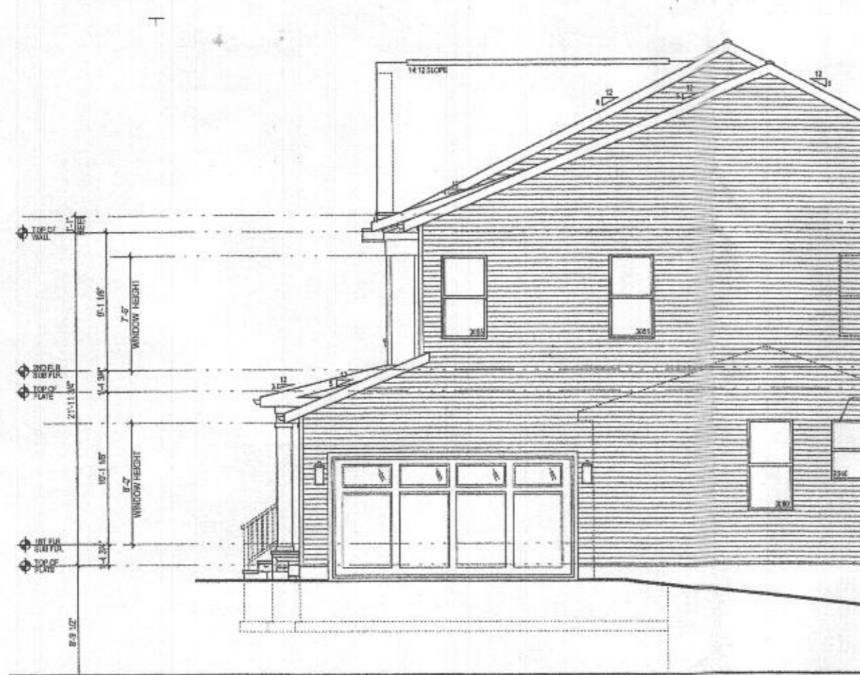
4 PART. RIGHT SIDE ELEVATION w/ OPT. 012 - SIDE LOAD GARAGE SCALE: 1/4"=1'-0" ELEV. 2 - SHOWN
