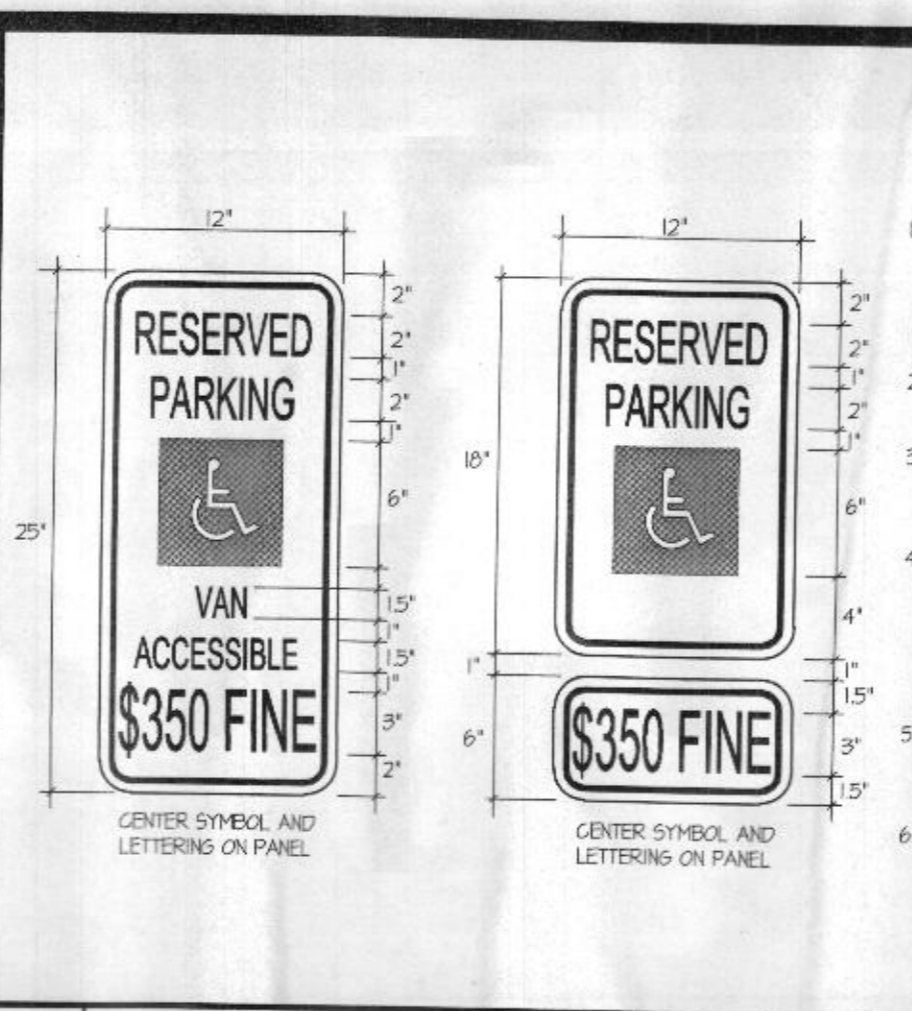
3 HANDICAP PARKING SIGNS DETAIL NO SCALE
