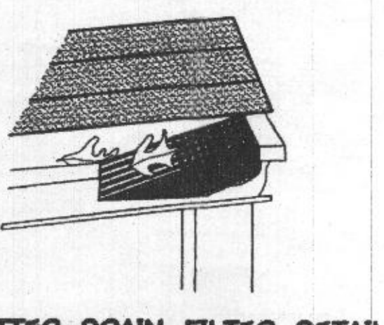
GUTTER DRAIN FILTER DETAIL NOT TO SCALE
