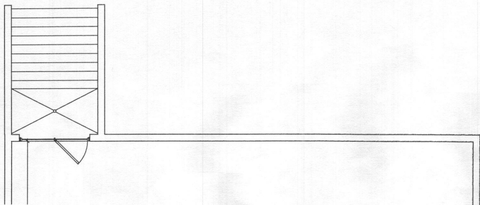
3 PARTIAL BASEMENT FLOOR PLAN SCALE: 1/4" = 1'-0" SHOWN W/ OPT. DOUBLE PATIO DOOR AREAWAY WELLED EXIT "DGG"
