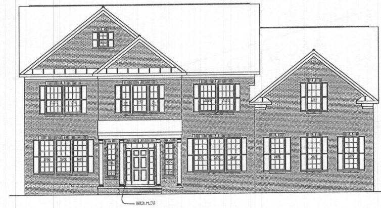
FRONT ELEVATION #1 (STANDARD BRICK) SCALE: 1/8" = 1'-0"
