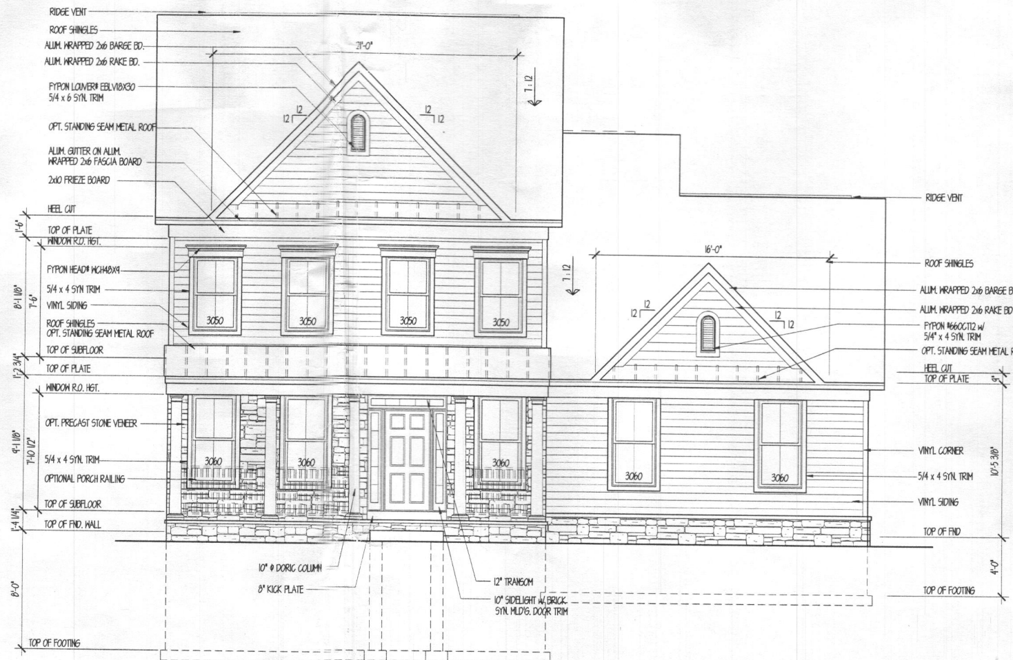
FRONT ELEVATION #2 W/ PRECAST STONE VENEER 1/4"=1'-0"
