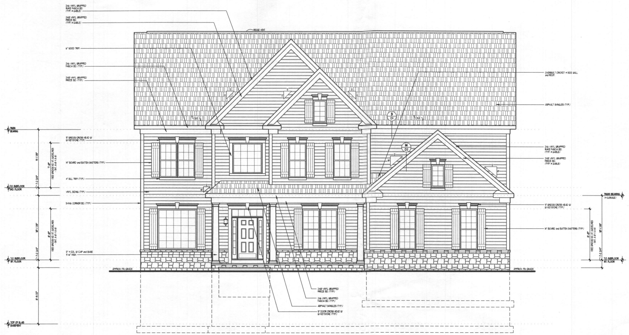
FRONT ELEVATION (STONE WATERTABLE and SIDING) SCALE: 1/4" = 1'-0"
