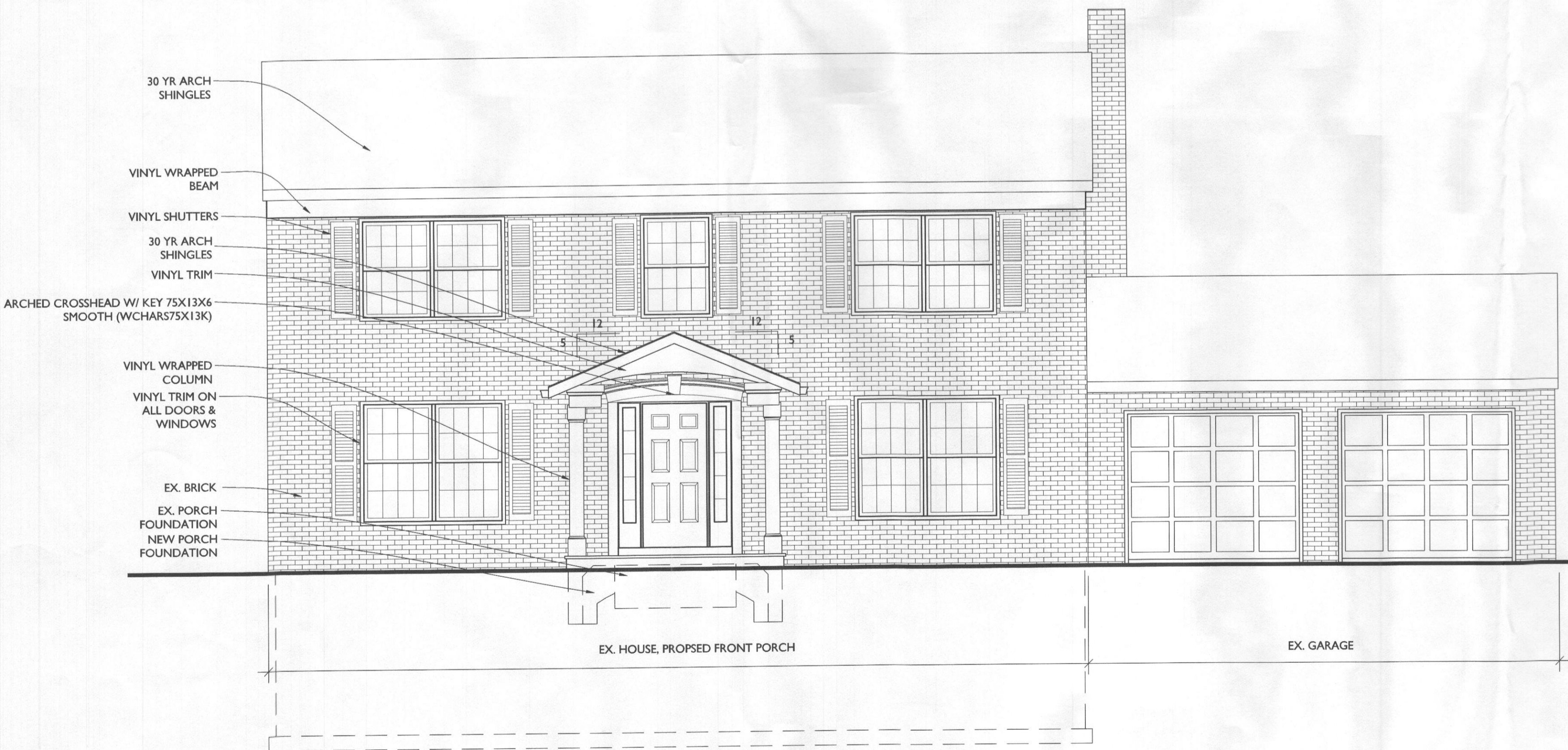
2 FRONT ELEVATION SCALE: 1/4"=1'-0"
