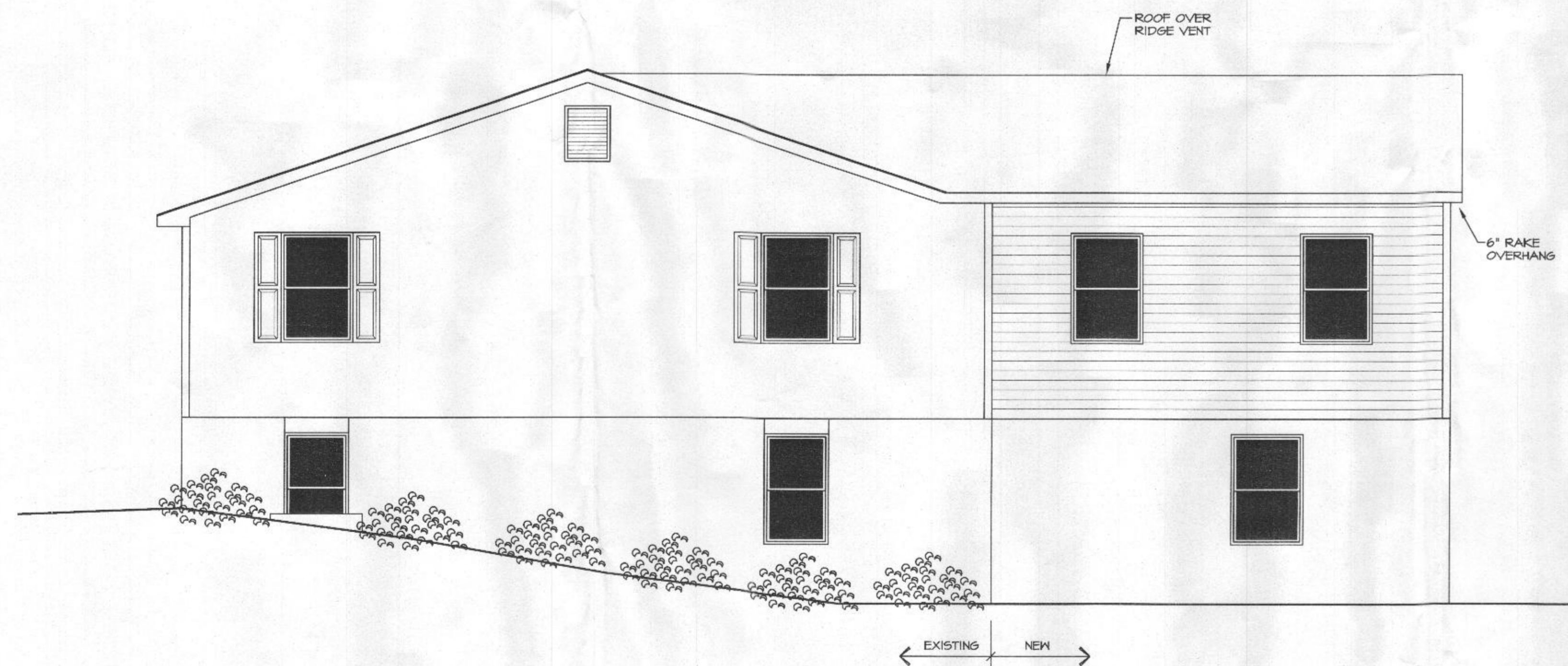
LEFT ELEVATION NEW CONSTRUCTION SCALE: 1/4" = 1'-0"
