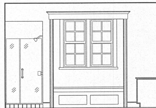
ID-1 Interior Elevation Master Bath 1/2" = 1'-0"
