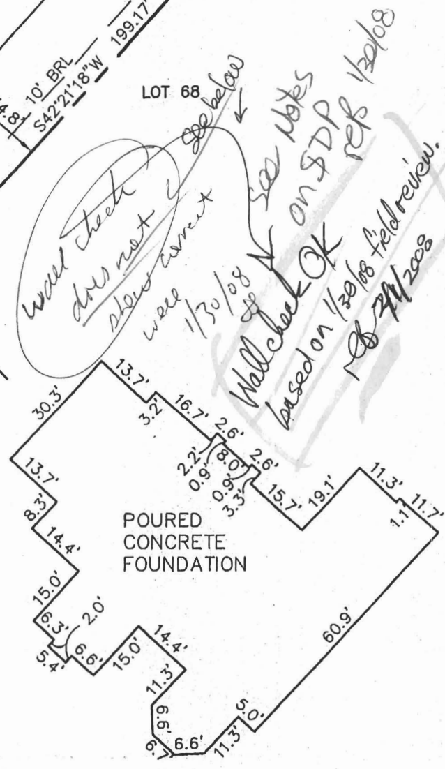
FOUNDATION DETAIL SCALE: 1" = 30'
