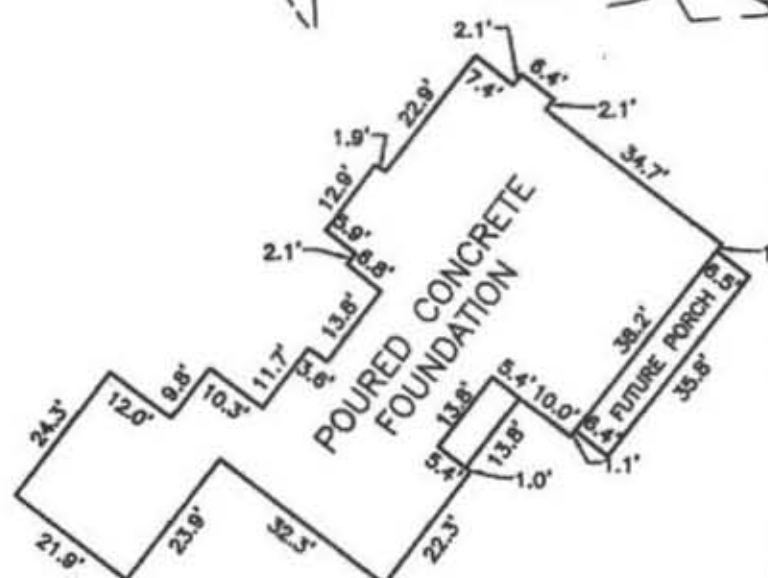
FOUNDATION DETAIL SCALE: 1" = 30'
