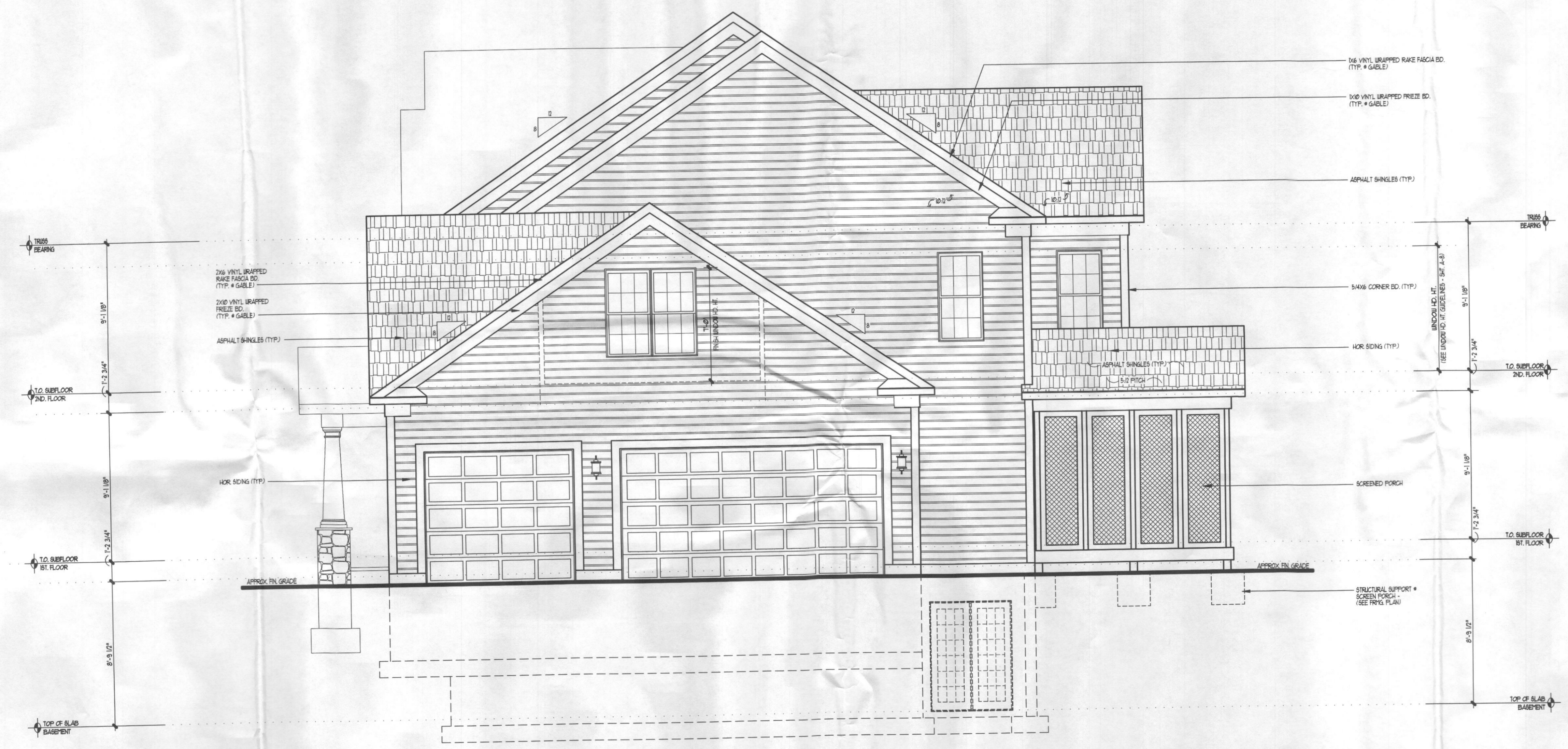
RIGHT SIDE ELEVATION (SIDING) SCALE: 1/4" = 1'-0"
