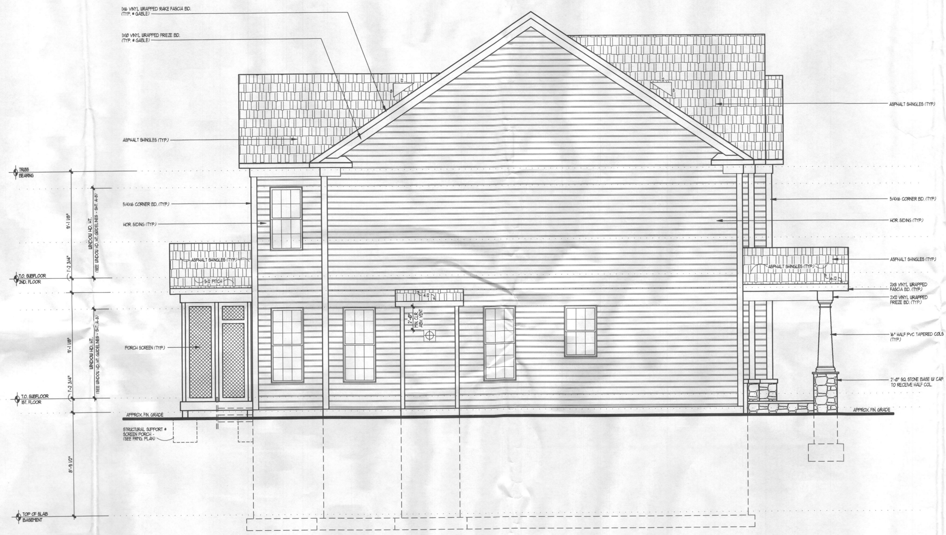
LEFT SIDE ELEVATION (SIDING) SCALE: 1/4" = 1'-0"
