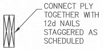
A1 TYPICAL MULTI PLY BEAM CONNECTION
