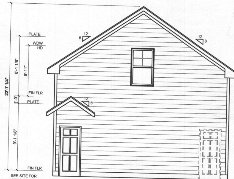
RIGHT SIDE ELEVATION - DETACHED GARAGE - A SCALE: 1/8"=1'-0"
