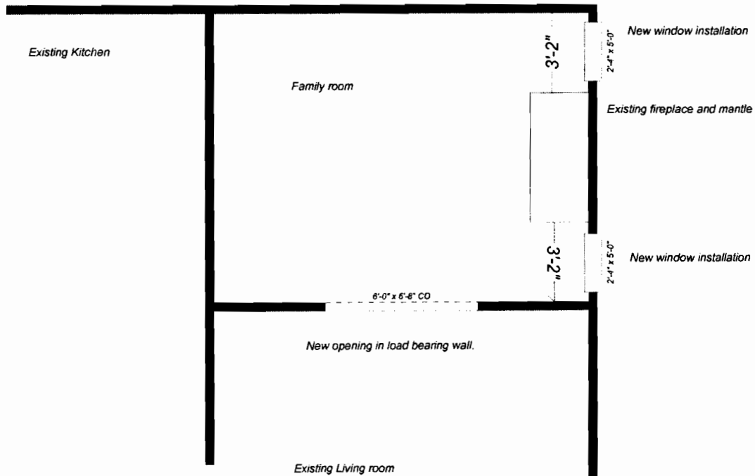
Floor plan with new window installation
